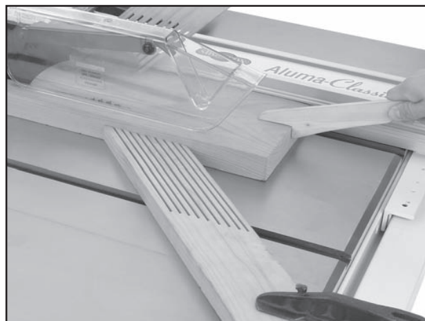
Figure 74. Typical ripping operation.
